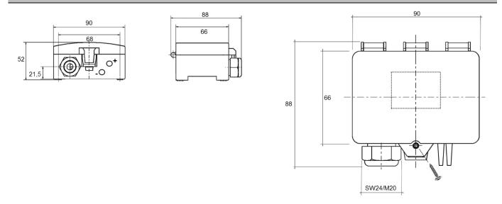
To gain protection IP 65 according to EN 60527 the cover has to be bolted at the prepared position, e.g. using a screw 3,5x10 mm according to EN 7981.
